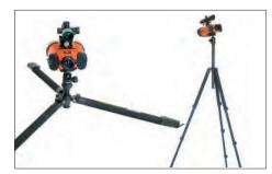
**Telescopic tripod** (comes as standard) Extended height up to 1.8m and comes with 3D attachment piece to orientate laser head in any direction. It integrates a hook underneath tripod top for hanging a ballast to ensure better stability.
