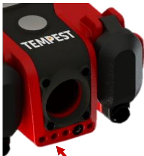
4 x charging contacts and charging plug
