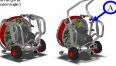
2) To close the carrying handle, unlock it using the index pin (ref. A).
