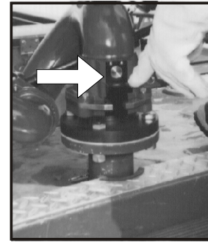
Figure 3.2.3 Slide bar locked, safety plunger is engaged.
