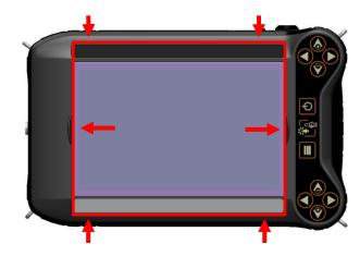
It is stored flat for easier transport. An elastic on its side is used to keep it flat and fix it to the control box. By placing it on the screen face, it protects the screen when moving around when the search device is not in use.
