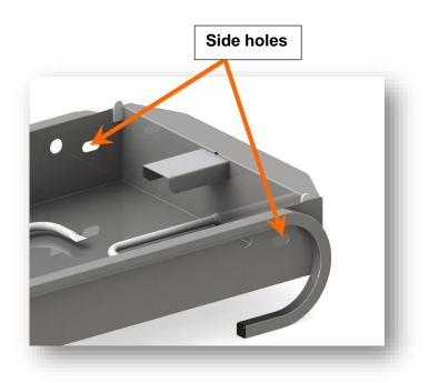
• Fill the tank until it overflows from the side holes.
