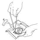
• Undo the screw in the centre of the pulley and remove the pulley. Insert and fasten a new starter cord to the pulley. Wind approx. 3 turns of the starter cord onto the pulley. Connect the pulley to the recoil spring so that the end of the spring engages in the pulley. Fit the screw in the centre of the pulley. Insert the starter cord through the hole in the starter housing and the starter handle. Make a secure knot in the end of the starter cord.
