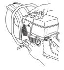
• Fit and tighten the screws that hold the starter.
