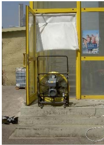
FIGURE 18: Stairs in front of the entrance. The figure shows that a large ventilator can even be placed very close to the door when a PathMaster ® is utilized. The PPV-method then becomes even more effective.
