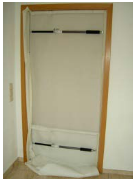
FIGURE 7: A) A second PathMaster® is fastened in the middle of a door. Smoke spread is limited even further, but access to the room is still possible. B) A second PathMaster® is fastened at the bottom of a door. There is practically no smoke spread possible – however, access to the room is also hindered.
