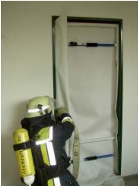
FIGURE 10: Utilizing two PathMasters® The second metal frame holds the fire proof curtain of the first PathMaster® in place. A nozzle can be used through the nearly closed opening; a very safe firefighting technique that avoids the introduction of fresh air (and oxygen!) into the fire area itself. This might also be used in wind influenced or wind driven fires.
