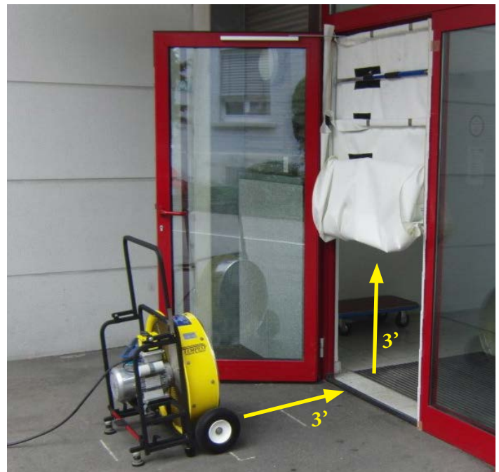
FIGURE 21: Using a PathMaster ® in the entrance door of a building increases the differential pressure and helps to show personnel present that this access is blocked by the fire department.
