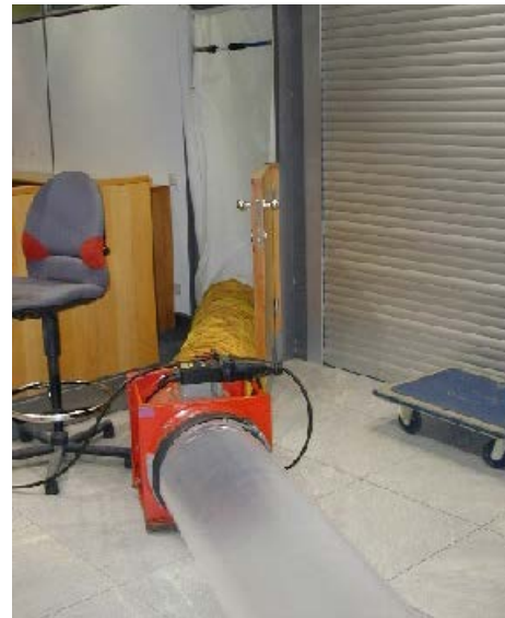
FIGURE 15: Room fire at an airport terminal in Stuttgart. To prevent smoke from spreading during the ventilation process, the door can be closed with a PathMaster®.
