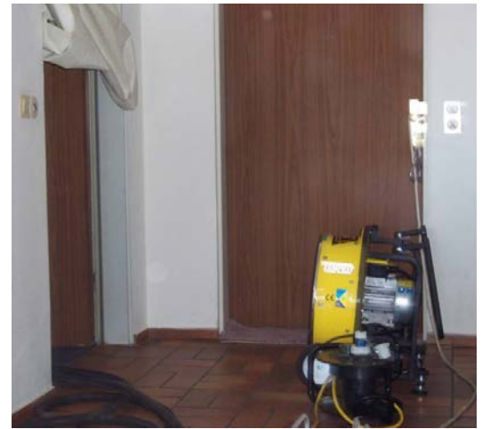
FIGURE 19: Corridor situation in a multi-story or high-rise building. The ventilator can be placed in an effective position in a small corridor in a building when the upper part of the entrance door is blocked with a PathMaster ®.
