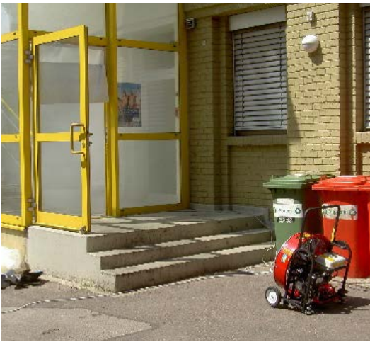
FIGURE 17: Stairs in front of the entrance. By utilizing a PathMaster ® in the upper part of the door (the lower part of the fire proof curtain is hung over the spreader bar of the metal frame), the PPV-method becomes more effective.
